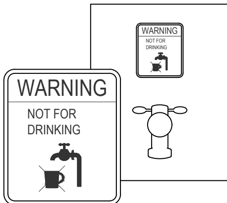
TYPICAL WARNING SIGN
