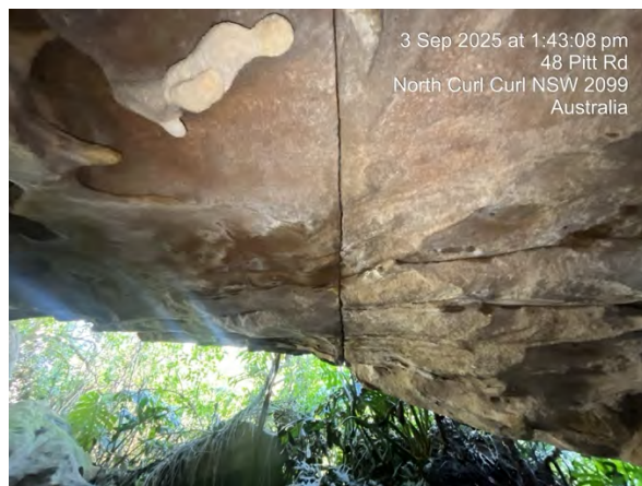
Photo 9: Vertical joint running ~N-S, approximately in line with the eastern boundary of the subject site.
