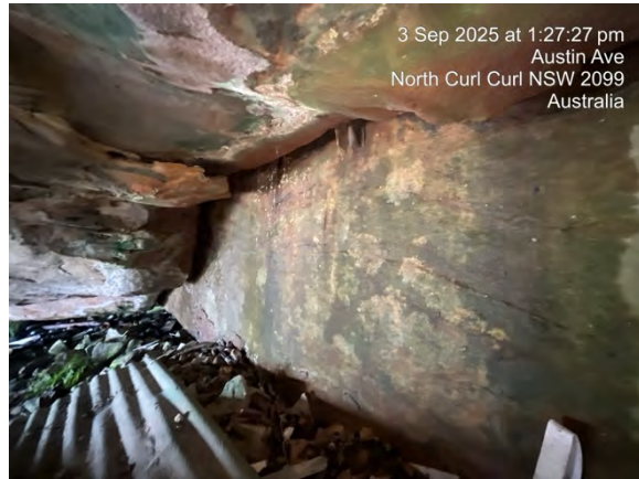
Photo 7: Significant vertical joint at the rear of the undercut bedrock running ~E-.
