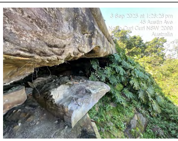
Photo 4: Undercut bedrock near rear boundary and historical block failure.
