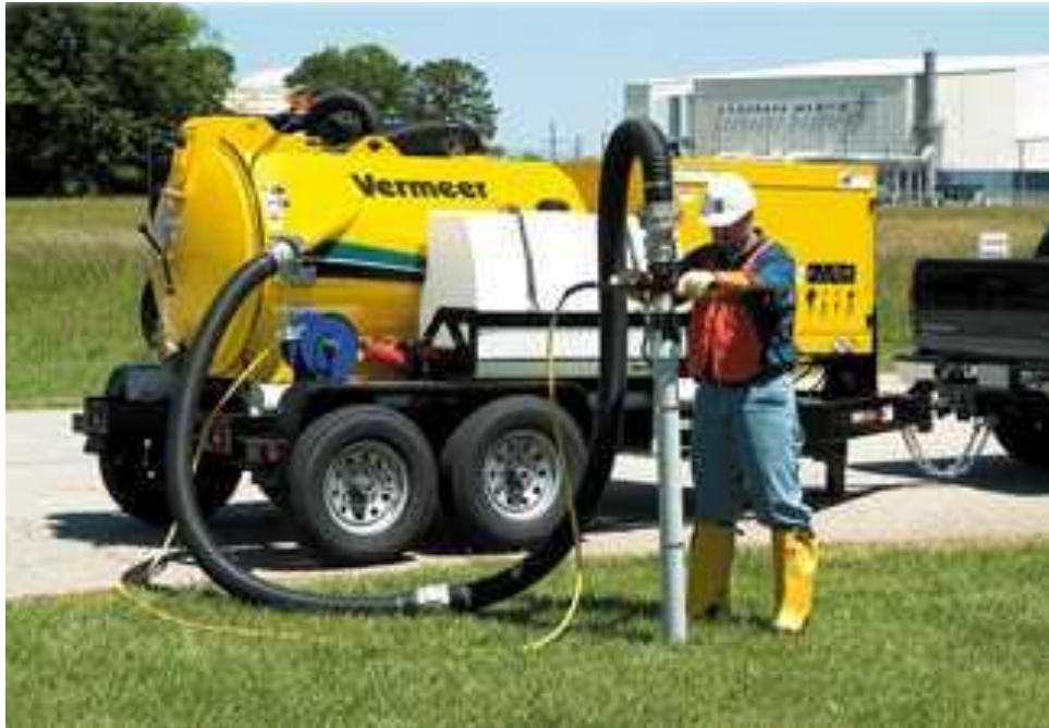
Figure 17 – Aero/Hydro vacuum excavator
