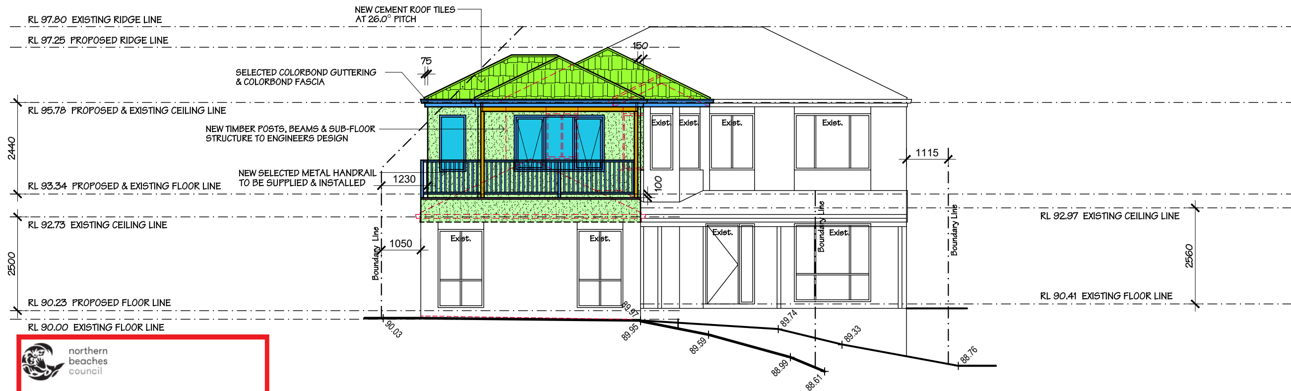
SOUTH-WESTERN ELEVATION - FRONT SCALE 1:100
