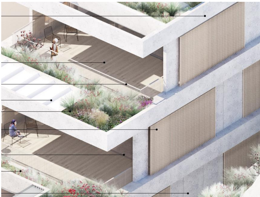
Figure 37 - vertical timber screens to window openings within the east and west side elevations
