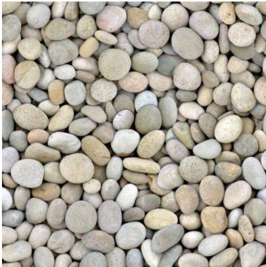
RIVERSTONE PEBBLE BALLAST TO CONCRETE ROOF
