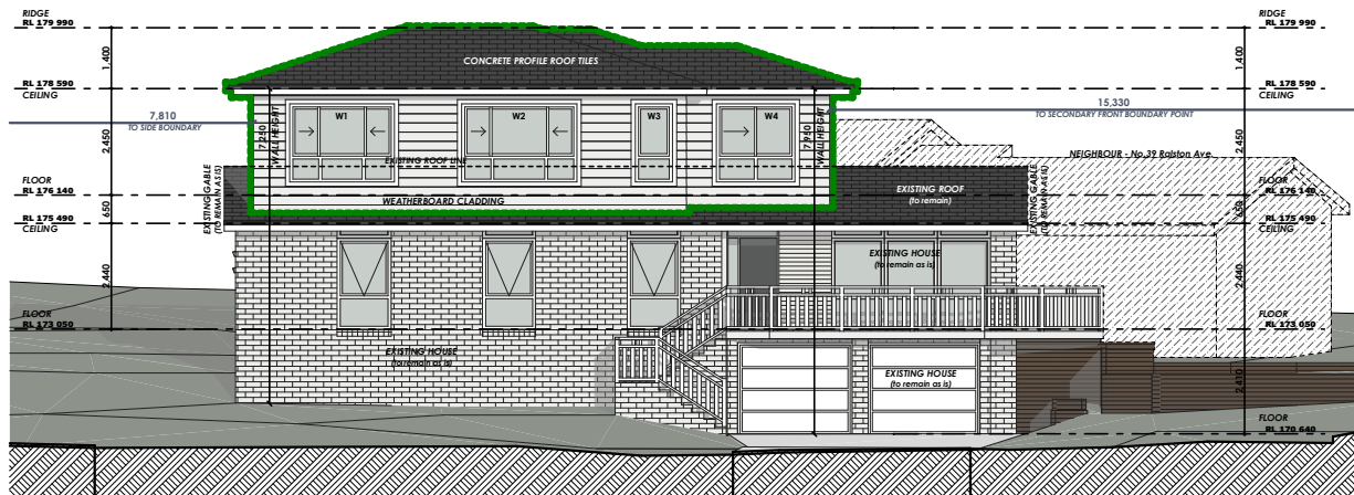
EAST ELEVATION (PRIMARY FRONT ELEVATION)
