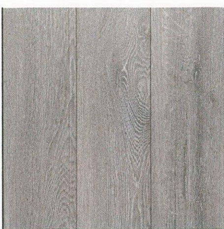
NATURALLY SILVERED TIMBER - TO FENCES AND OPEN CARPORT STRUCTURE
