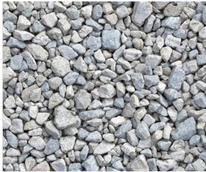
CONCRETE ROOF BALAST RIVER PEBBLE
