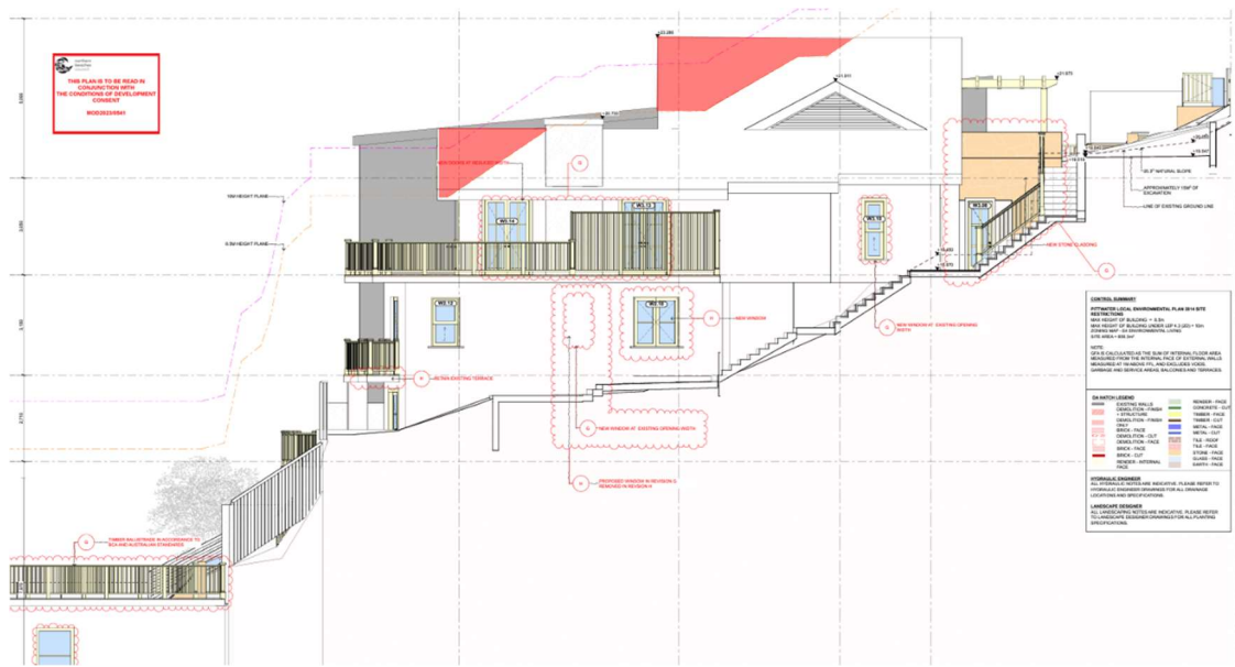
Figure 6 – Extract of the Approved Plans for 961 Barrenjoey Road, with exceedance of 8.5m (to assumed ground) shown in red Source: Northern Beaches Council DA Tracker
