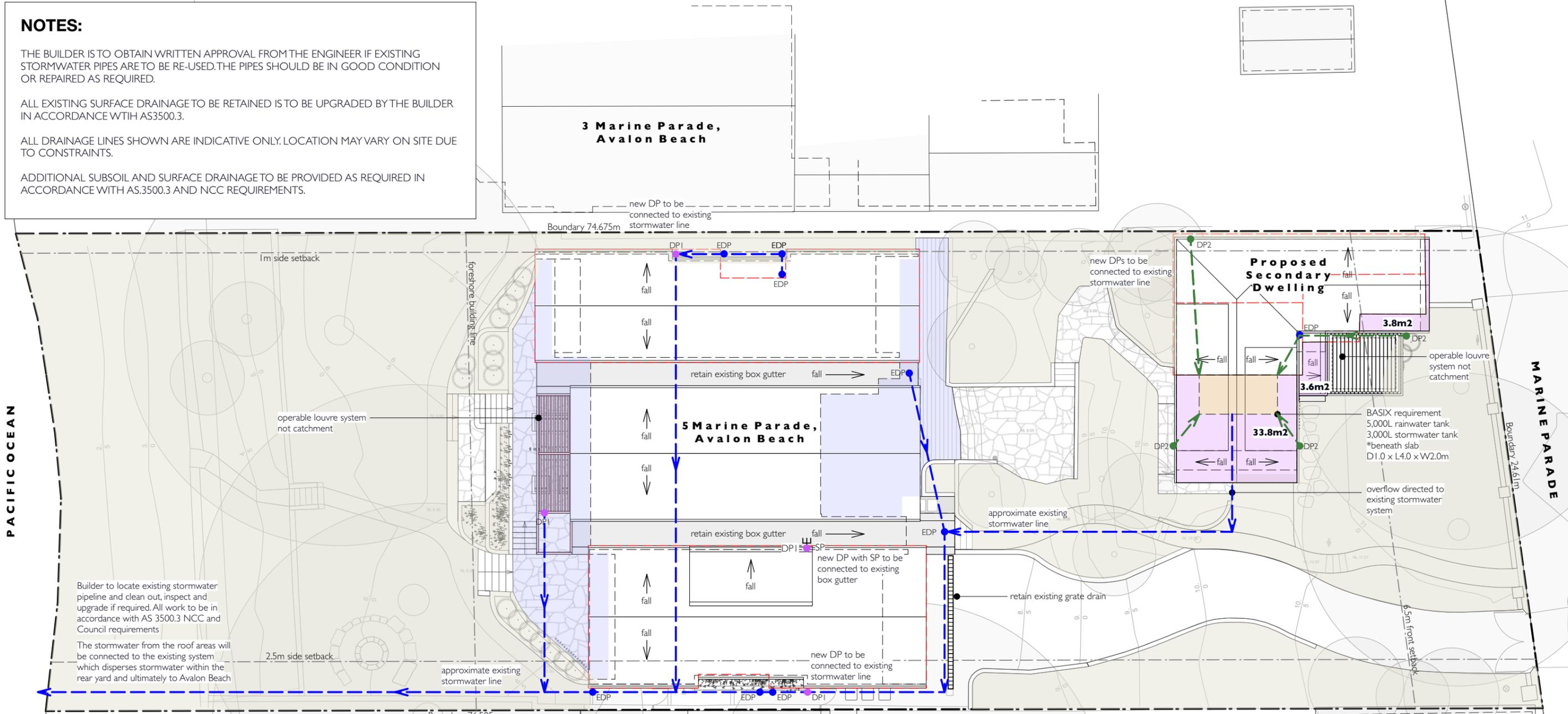
Builder to locate existing stormwater pipeline and clean out, inspect and upgrade if required. All work to be in accordance with AS 3500.3 NCC and Council requirements
