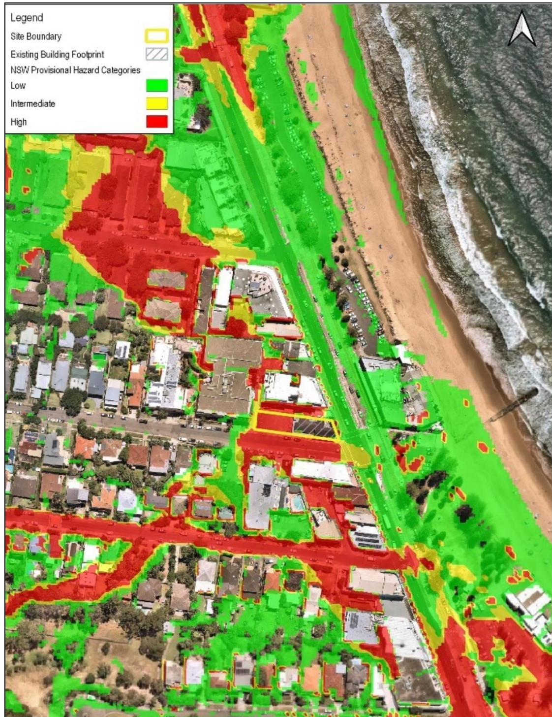
Figure 10. PMF Provisional Hazard – Existing Conditions
