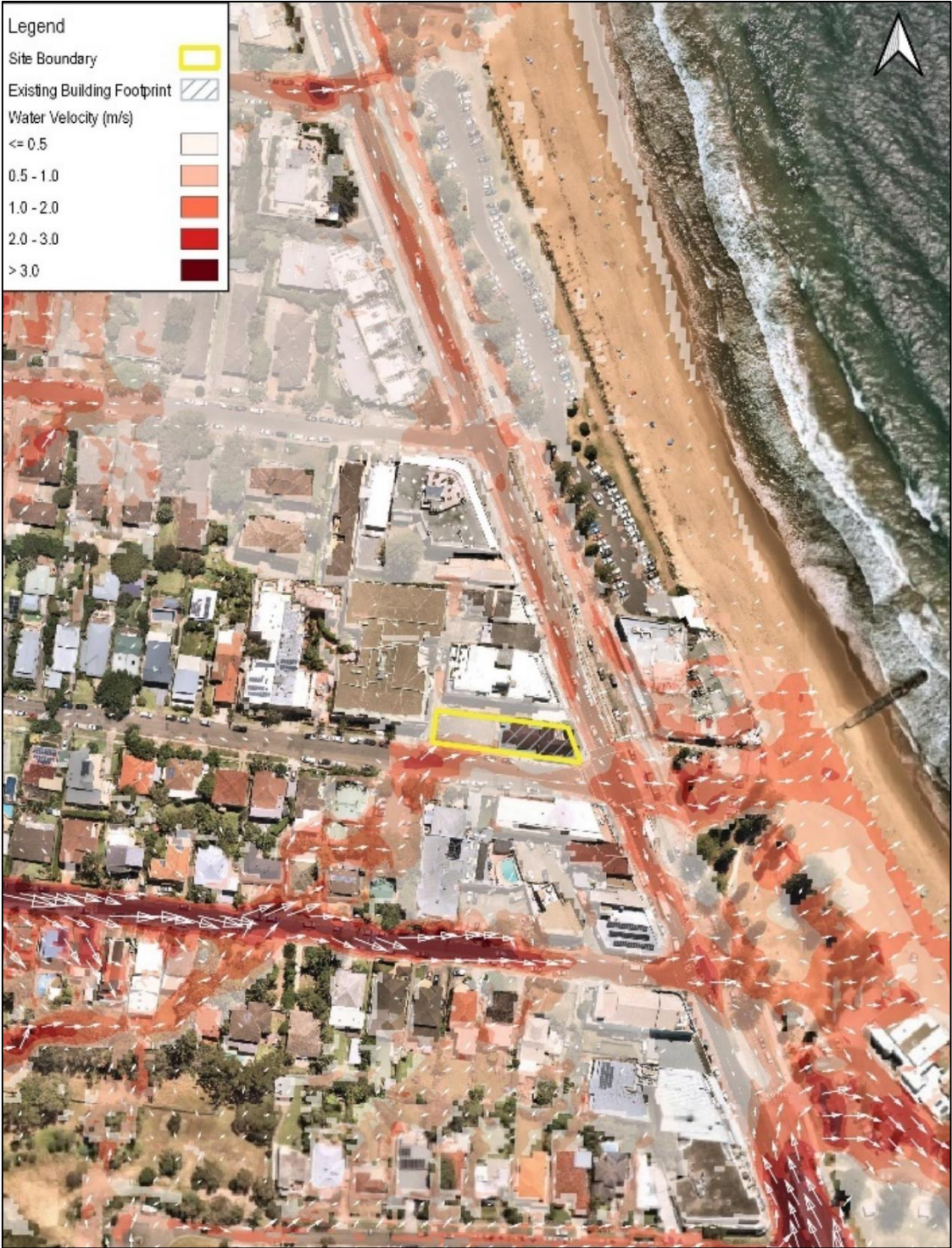
Figure 9. PMF Water Velocity – Existing Conditions
