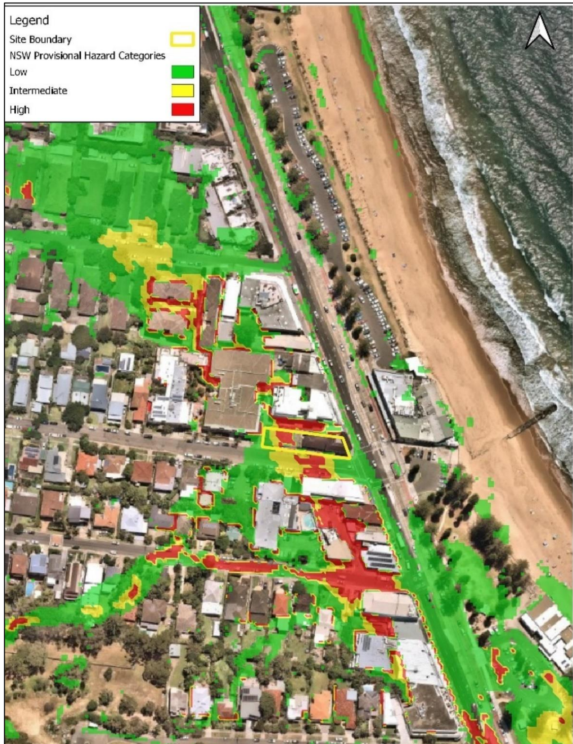
Figure 13. 1%AEP Provisional Hazard – Proposed Conditions
