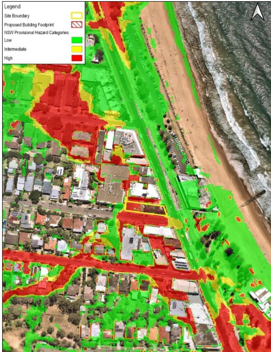
Figure 16. PMF Provisional Hazard – Proposed Conditions
