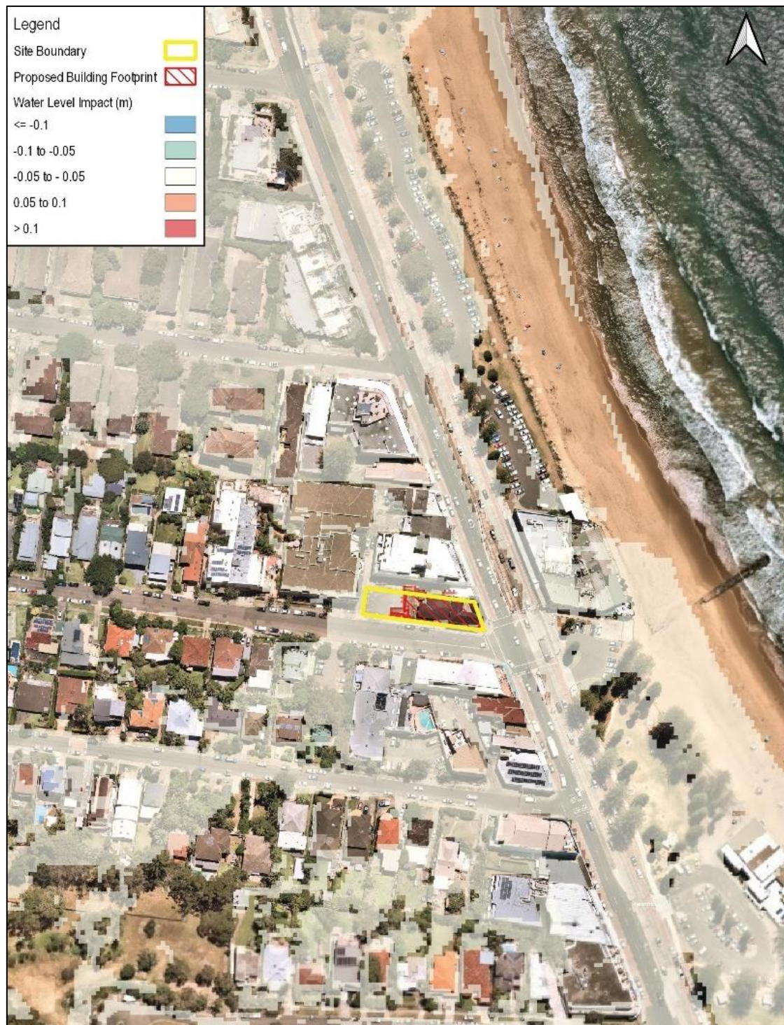
Figure 18. PMF Water Level Impact
