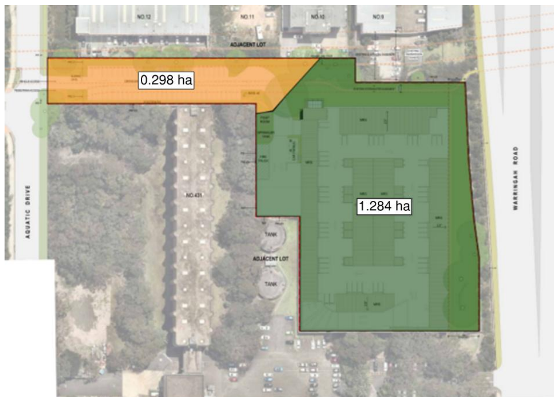
Figure 4.2 – Development Catchment Areas (Green refers to stormwater quantity and quality catchment, Orange refers to bypass catchment)
