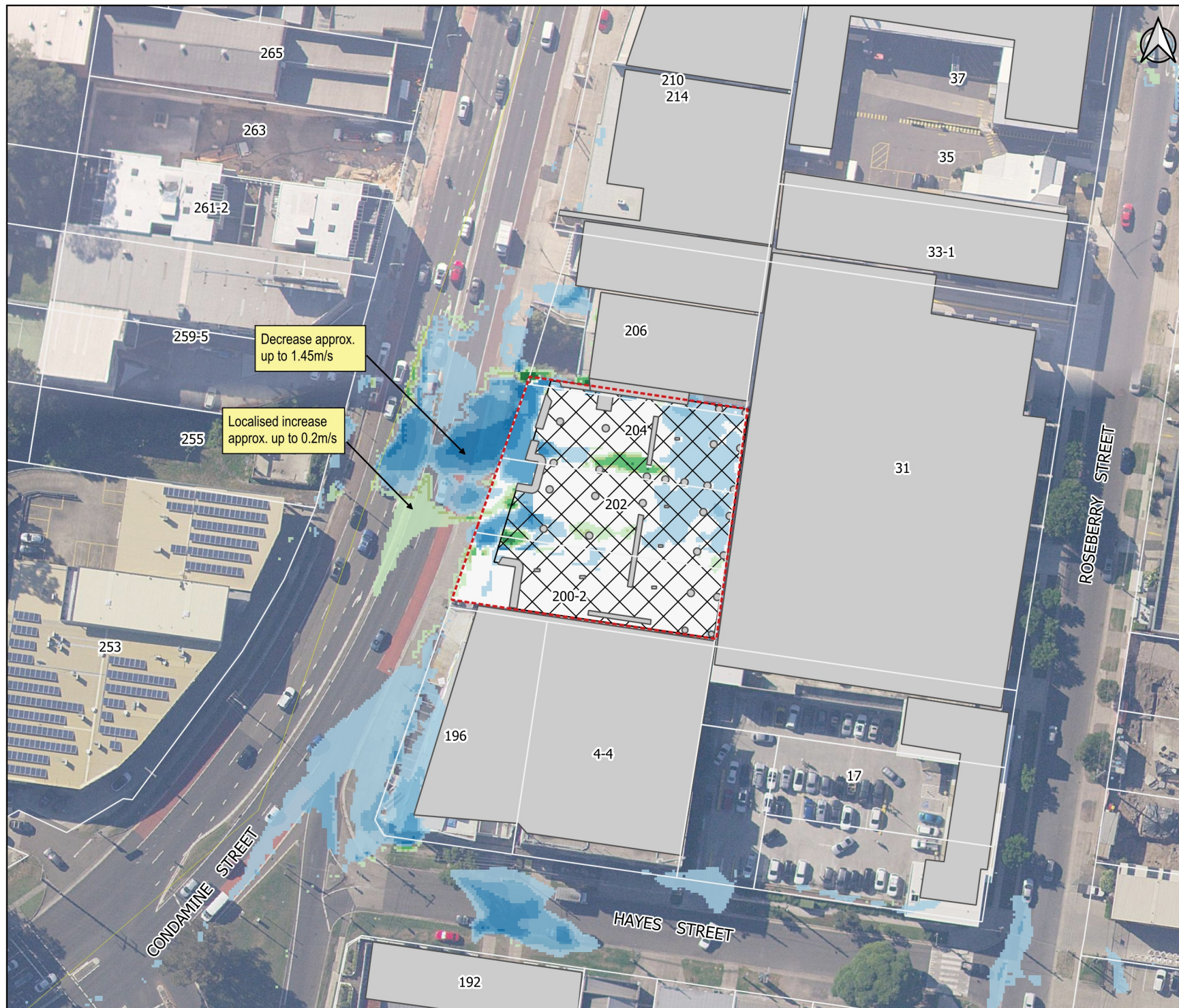
Figure C4[A] 1% AEP Flood Velocity Difference Developed minus Existing
