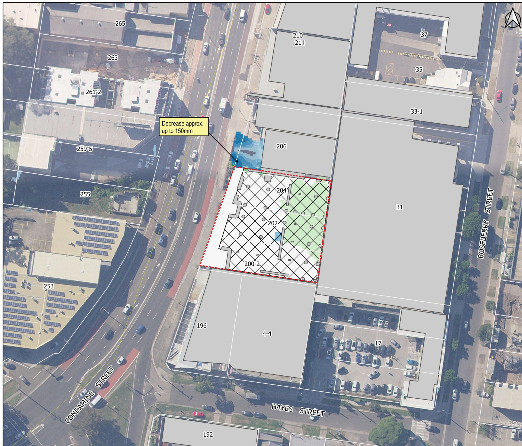
Figure C1[A] 20% AEP Flood Elevation Difference Developed minus Existing
