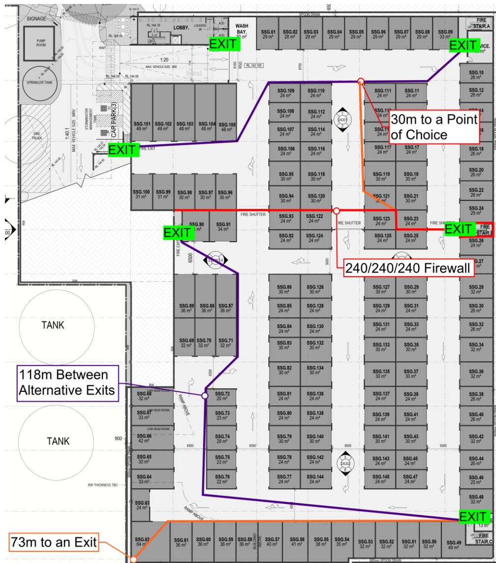
Figure 6-3: Ground Floor Extended Travel Distances
